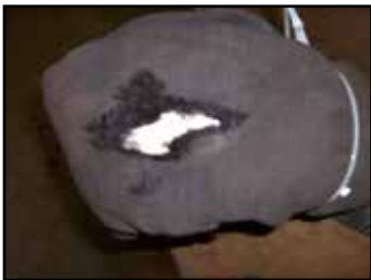
Exposed load bearing yarns
