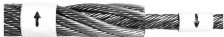
Alternate Lay – Alternating right regular and right lang lay strands.
