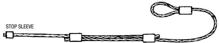
LAP SPLICE - OVAL SLEEVES OR DUPLEX
