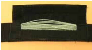
Velcro inspection window
